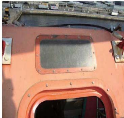
Glass not clear – poor visibility
