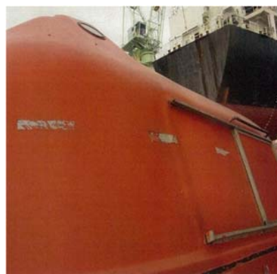
Deteriorated. reflective tape
