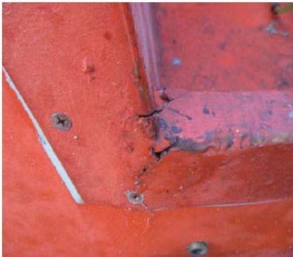
Damaged lifeboat side shell
