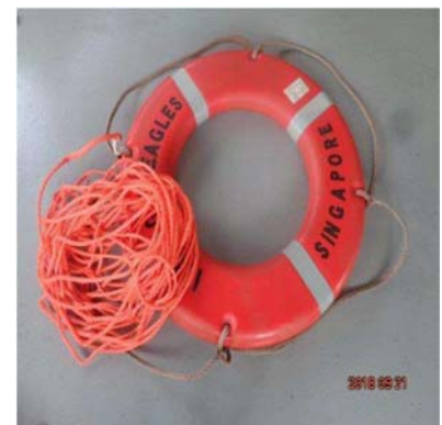
Buoyant lines not of non-kinking type
