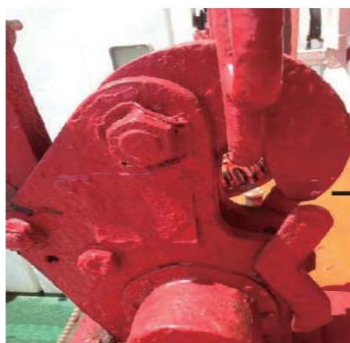
Onload release seized due to excessive paint
