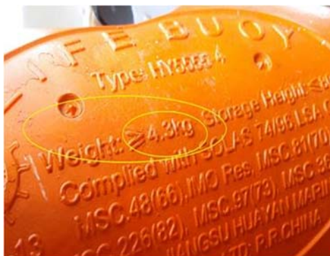
Bridge wing lifebuoys not weighing at least 4.0 KG to operate the quick release arrangement
