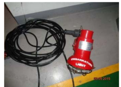
Forward liferaft portable emergency light not operational
