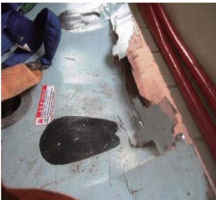
Damaged lifeboat seat
